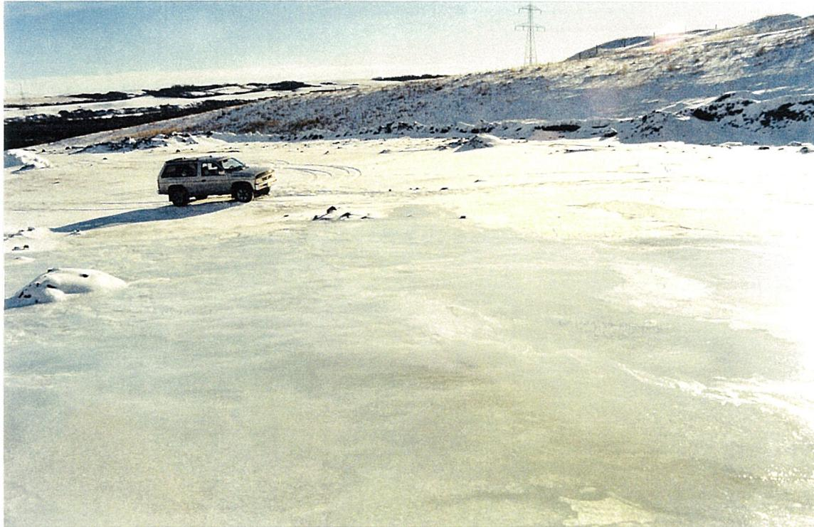
Fig. 6. Looking east from the underpass in February 1997. Ice buildup from groundwater seeping from the intertill gravel and surficial sand.
