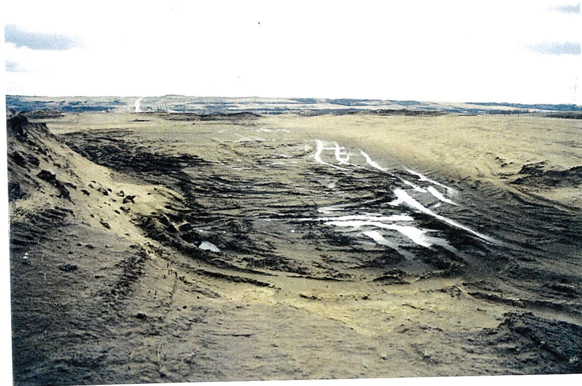
Fig. 22. Unstable ground in wet areas where head in the surficial sand is near the ground surface west of the underpass structure in early May 1997.
